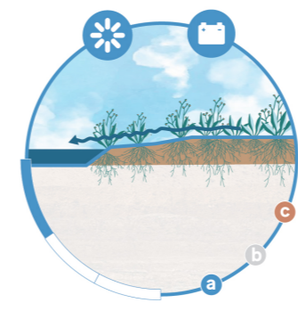
w10 Use existing height differences to design water runoff: organise your water storage at the lowest point.
