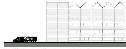
1. The Carlsberg Brewery is demolished and afterwards, the Copenhagen Metro removes temporary structures such as scaffolding.
